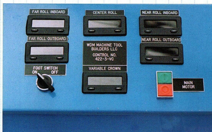
Variable crown position is indicated via electronic digital readout. See photograph above.
