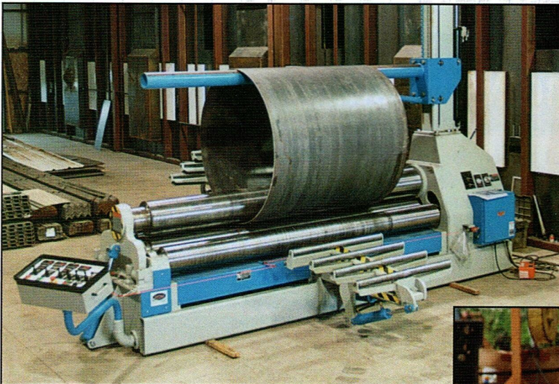
403-12-10 (1/2" x 10') with side and overhead supports, swinging console control and 423-LP-6 control used for process and dust collection equipment.
