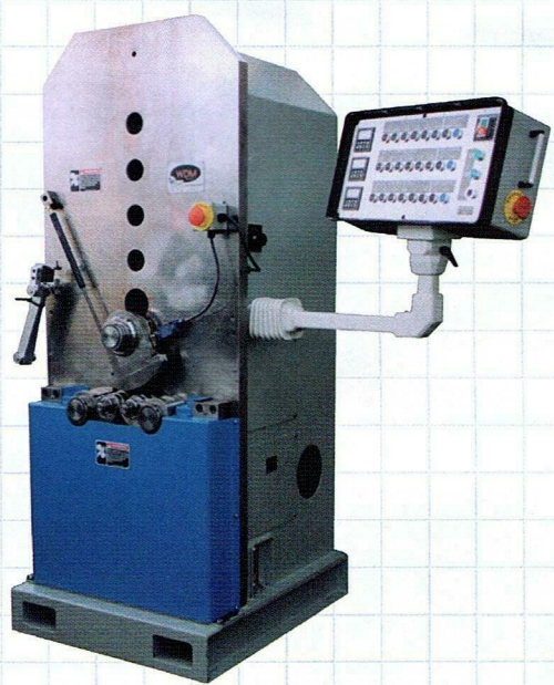
Machine to form titanium pins used for hip replacements.
