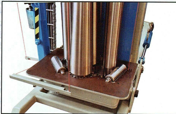
Special automatic cone roll for rolling concrete mixer drum sections. Patent pending.
