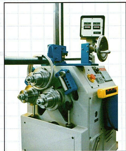
AR-20 with manually operated overhead support, DRO, and pendant control, spiral rolling stainless steel tube.
