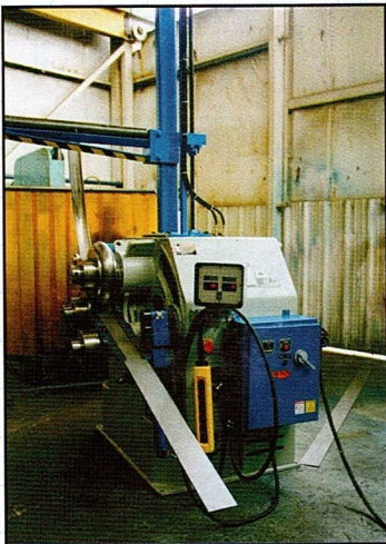
AR-40 with overhead support forming stainless steel half pipes in one pass.
