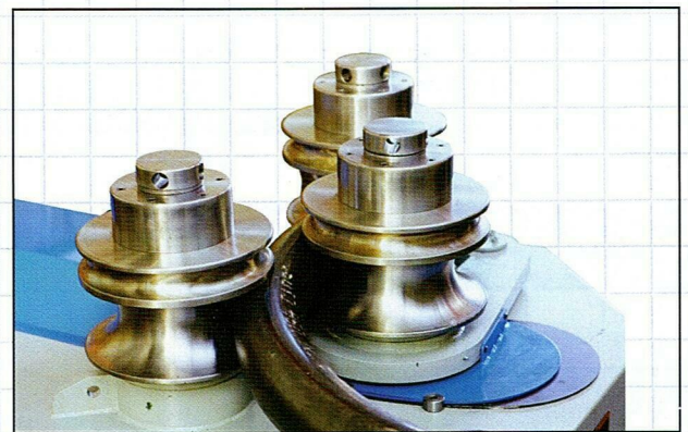
Pipe dies on PSPR-61 Section Roll (no guide rolls) rolling a large pipe section.
