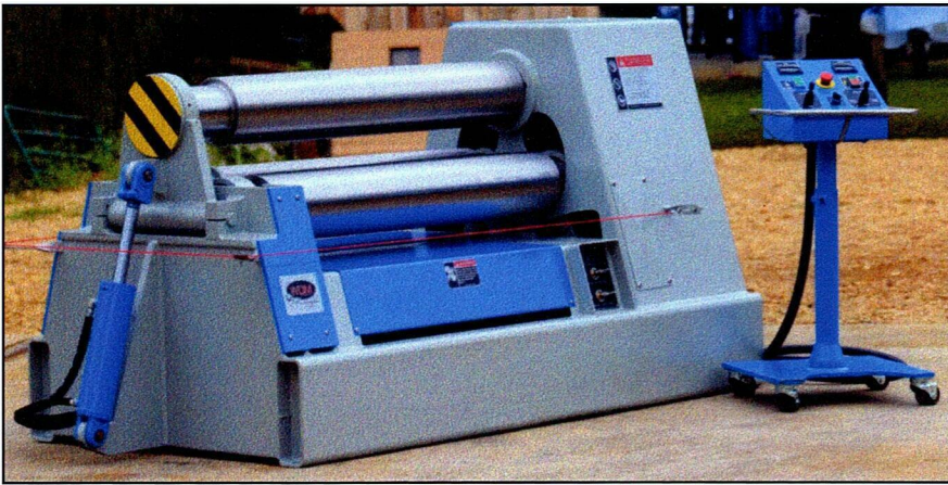
101-8-4 Plate Roll w/Rolling Console Control
